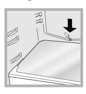
water is ducted to the back of the appliance by a special discharge outlet (see diagram) where the heat produced by the compressor causes it to evaporate. It is necessary to clean the discharge hole regularly so that the water can flow out easily.
